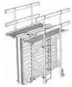
Figure 27; Steel wall form ( www.joostdevree.nl )
